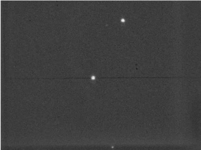
Figure 4: Test frame of the guiding camera. AU Ser is positioned directly on the slit.
